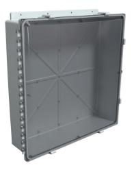
AttaBox Heartland SL series enclosure, NEMA 1/3R/4/4X/12, 24 x 24 x 6in (HxWxD), wall mount, polycarbonate, Pantone 7541 C light gray, smoked polycarbonate single-door, polycarbonate quick-release latch.
