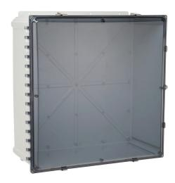
AttaBox Heartland series enclosure, NEMA 1/3R/4/4X/12,  $24 \times 24 \times 10$  in (HxWxD), wall mount, polycarbonate, Pantone 7541 C light gray, smoked polycarbonate single-door, stainless steel quick-release latch.
