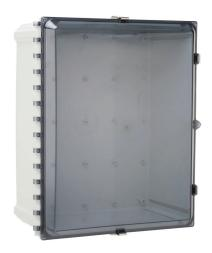
AttaBox Heartland series enclosure, NEMA 1/3R/4/4X/12, 20 x 16 x 8in (HxWxD), wall mount, polycarbonate, Pantone 7541 C light gray, smoked polycarbonate single-door, stainless steel quick-release latch.
