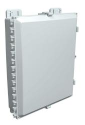
AttaBox Heartland SL series enclosure, NEMA 1/3R/4/4X/12, 20 x 16 x 4in (HxWxD), wall mount, polycarbonate, Pantone 7541 C light gray, single-door, polycarbonate quick-release latch.
