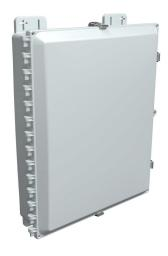
AttaBox Heartland SL series enclosure, NEMA 1/3R/4/4X/12, 20 x 16 x 4in (HxWxD), wall mount, polycarbonate, Pantone 7541 C light gray, single-door, stainless steel quick-release latch.
