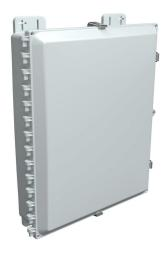
AttaBox Heartland SL series enclosure, NEMA 1/3R/4/4X/12, 20 x 16 x 4in (HxWxD), wall mount, polycarbonate, Pantone 7541 C light gray, single-door, stainless steel quick-release latch.
