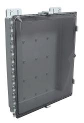
AttaBox Heartland SL series enclosure, NEMA 1/3R/4/4X/12, 20 x 16 x 4in (HxWxD), wall mount, polycarbonate, Pantone 7541 C light gray, smoked polycarbonate single-door, polycarbonate quick-release latch.
