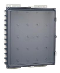
AttaBox Heartland SL series enclosure, NEMA 1/3R/4/4X/12, 18 x 16 x 4in (HxWxD), wall mount, polycarbonate, Pantone 7541 C light gray, smoked polycarbonate single-door, polycarbonate quick-release latch.
