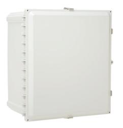
AttaBox Heartland series enclosure, NEMA 1/3R/4/4X/12, 18 x 16 x 10in (HxWxD), wall mount, polycarbonate, Pantone 7541 C light gray, single-door, stainless steel quick-release latch.
