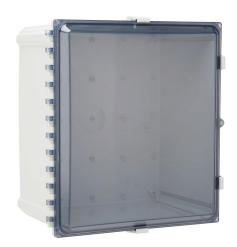
AttaBox Heartland series enclosure, NEMA 1/3R/4/4X/12,  $18 \times 16 \times 10$  in (HxWxD), wall mount, polycarbonate, Pantone 7541 C light gray, smoked polycarbonate single-door, polycarbonate quick-release latch.
