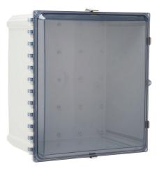
AttaBox Heartland series enclosure, NEMA 1/3R/4/4X/12, 18 x 16 x 10in (HxWxD), wall mount, polycarbonate, Pantone 7541 C light gray, smoked polycarbonate single-door, stainless steel quick-release latch.
