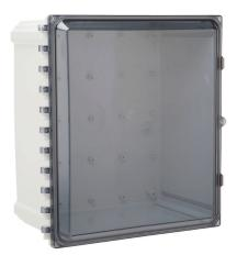
AttaBox Heartland series enclosure, NEMA 1/3R/4/4X/12, 16 x 14 x 8in (HxWxD), wall mount, polycarbonate, Pantone 7541 C light gray, smoked polycarbonate single-door, stainless steel quick-release latch.
