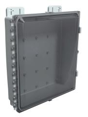
AttaBox Heartland SL series enclosure, NEMA 1/3R/4/4X/12, 16 x 14 x 4in (HxWxD), wall mount, polycarbonate, Pantone 7541 C light gray, smoked polycarbonate single-door, polycarbonate quick-release latch.
