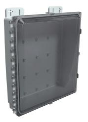
AttaBox Heartland SL series enclosure, NEMA 1/3R/4/4X/12, 16 x 14 x 4in (HxWxD), wall mount, polycarbonate, Pantone 7541 C light gray, smoked polycarbonate single-door, stainless steel quick-release latch.
