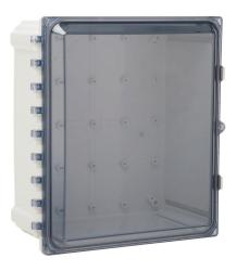
AttaBox Heartland series enclosure, NEMA 1/3R/4/4X/12, 14 x 12 x 6in (HxWxD), wall mount, polycarbonate, Pantone 7541 C light gray, smoked polycarbonate single-door, stainless steel quick-release latch.
