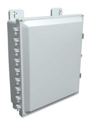
AttaBox Heartland SL series enclosure, NEMA 1/3R/4/4X/12, 14 x 12 x 4in (HxWxD), wall mount, polycarbonate, Pantone 7541 C light gray, single-door, stainless steel quick-release latch.
