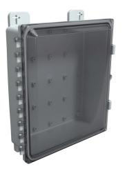
AttaBox Heartland SL series enclosure, NEMA 1/3R/4/4X/12, 14 x 12 x 4in (HxWxD), wall mount, polycarbonate, Pantone 7541 C light gray, smoked polycarbonate single-door, polycarbonate quick-release latch.
