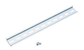
AttaBox DIN rail, slotted, 35mm width, 7mm height, 10.8in length, plated steel. For use with AHxx1210xxxx and AHxx1412xxxx Heartland series enclosures.
