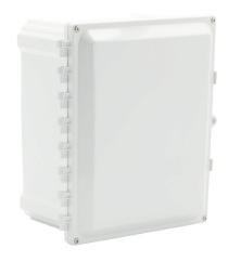
AttaBox Heartland series enclosure, NEMA 1/3R/4/4X/6P/12,  $12 \times 10 \times 6$ in (HxWxD), wall mount, polycarbonate, Pantone 7541 C light gray, hinged screw cover.
