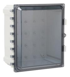
AttaBox Heartland series enclosure, NEMA 1/3R/4/4X/12,  $12 \times 10 \times 6in$  (HxWxD), wall mount, polycarbonate, Pantone 7541 C light gray, smoked polycarbonate single-door, polycarbonate quick-release latch.
