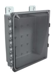
AttaBox Heartland SL series enclosure, NEMA 1/3R/4/4X/12, 12 x 10 x 4in (HxWxD), wall mount, polycarbonate, Pantone 7541 C light gray, smoked polycarbonate single-door, stainless steel quick-release latch.
