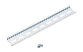
AttaBox DIN rail, slotted, 35mm width, 7mm height, 8.9in length, plated steel. For use with AHx108xxxx, AHxx1010xxxx and AHxx1210xxxx Heartland series enclosures.
