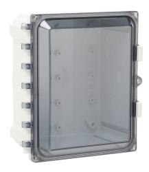
AttaBox Heartland series enclosure, NEMA 1/3R/4/4X/12,  $10 \times 8 \times 4$  in (HxWxD), wall mount, polycarbonate, Pantone 7541 C light gray, smoked polycarbonate single-door, polycarbonate quick-release latch.
