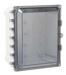
AttaBox Heartland series enclosure, NEMA 1/3R/4/4X/12,  $10 \times 8 \times 4$  in (HxWxD), wall mount, polycarbonate, Pantone 7541 C light gray, smoked polycarbonate single-door, stainless steel quick-release latch.
