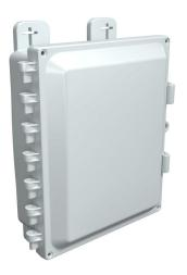
AttaBox Heartland SL series enclosure, NEMA 1/3R/4/4X/12, 10 x 8 x 3in (HxWxD), wall mount, polycarbonate, Pantone 7541 C light gray, single-door, polycarbonate quick-release latch.
