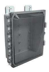
AttaBox Heartland SL series enclosure, NEMA 1/3R/4/4X/12,  $10 \times 8 \times 3$  in (HxWxD), wall mount, polycarbonate, Pantone 7541 C light gray, smoked polycarbonate single-door, polycarbonate quick-release latch.
