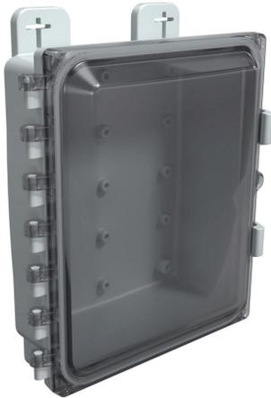
AttaBox Heartland SL series enclosure, NEMA 1/3R/4/4X/12, 10 x 8 x 3in (HxWxD), wall mount, polycarbonate, Pantone 7541 C light gray, smoked polycarbonate single-door, polycarbonate quick-release latch.
