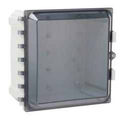
AttaBox Heartland series enclosure, NEMA 1/3R/4/4X/12, 10 x 10 x 6in (HxWxD), wall mount, polycarbonate, Pantone 7541 C light gray, smoked polycarbonate single-door, polycarbonate quick-release latch.
