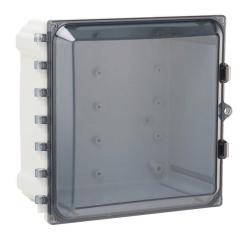
AttaBox Heartland series enclosure, NEMA 1/3R/4/4X/12, 10 x 10 x 6in (HxWxD), wall mount, polycarbonate, Pantone 7541 C light gray, smoked polycarbonate single-door, stainless steel quick-release latch.
