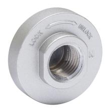
NITRA pneumatic gauge port adapter plate, 1/4in female NPT connection(s), aluminum. For use with Ax-4 and Ax-6 series air prep components. (3) o-rings included.
