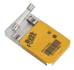
Bussmann fuse, AGC series, small dimension, fast-acting, 8A, 250 VAC, glass tube. Package of 5. Supplemental, electronic protection applications. Manufacturer part number: AGC-8-R.
