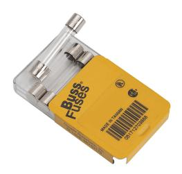
Bussmann fuse, AGC series, small dimension, fast-acting, 4A, 250 VAC, glass tube. Package of 5. Supplemental, electronic protection applications. Manufacturer part number: AGC-4-R.
