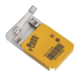
Bussmann fuse, AGC series, small dimension, fast-acting, 2A, 250 VAC, glass tube. Package of 5. Supplemental, electronic protection applications. Manufacturer part number: AGC-2-R.
