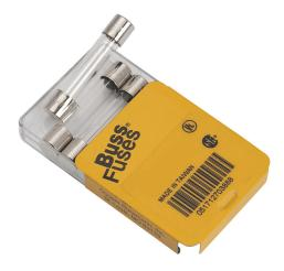
Bussmann fuse, AGC series, small dimension, fast-acting, 2.5A, 250 VAC, glass tube. Package of 5. Supplemental, electronic protection applications. Manufacturer part number: AGC-2-1/2-R.
