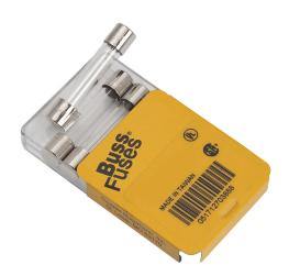
Bussmann fuse, AGC series, small dimension, fast-acting, 15A, 32 VAC, glass tube. Package of 5. Supplemental, electronic protection applications. Manufacturer part number: AGC-15-R.
