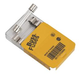
Bussmann fuse, AGC series, small dimension, fast-acting, 1.5A, 250 VAC, glass tube. Package of 5. Supplemental, electronic protection applications. Manufacturer part number: AGC-1-1/2-R.
