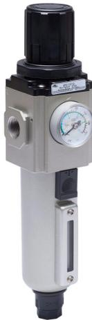
NITRA pneumatic filter-regulator, 3/8in female NPT inlet(s), 3/8in female NPT outlet(s), 20-130 psi adjustable range, manual/semi-automatic drain, die-cast aluminum bowl, sight gauge. For use with Ax-33 series air prep components.
