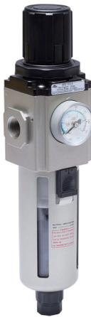
NITRA pneumatic filter-regulator, 3/8in female NPT inlet(s), 3/8in female NPT outlet(s), 20-130 psi adjustable range, automatic drain, polycarbonate bowl, bowl guard. For use with Ax-33 series air prep components.
