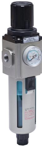
NITRA pneumatic filter-regulator, 1/4in female NPT inlet(s), 1/4in female NPT outlet(s), 20-130 psi adjustable range, automatic drain, nylon bowl, bowl guard. For use with Ax-32 series air prep components.
