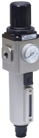
NITRA pneumatic filter-regulator, 1/4in female NPT inlet(s), 1/4in female NPT outlet(s), 20-60 psi adjustable range, manual/semi-automatic drain, die-cast aluminum bowl, sight gauge. For use with Ax-32 series air prep components.
