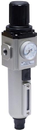
NITRA pneumatic filter-regulator, 1/4in female NPT inlet(s), 1/4in female NPT outlet(s), 20-60 psi adjustable range, automatic drain, die-cast aluminum bowl, sight gauge. For use with Ax-32 series air prep components.
