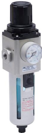
NITRA pneumatic filter-regulator, 1/8in female NPT inlet(s), 1/8in female NPT outlet(s), 20-60 psi adjustable range, manual/semi-automatic drain, nylon bowl, bowl guard. For use with Ax-21 series air prep components.
