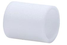
NITRA particulate filter element, replacement, 40 micron particles, high-density polyethylene (HDPE). For use with AF-2 series filters or AFR-2 series filter regulators.
