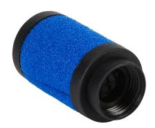
NITRA coalescing oil removal filter element, replacement, 0.3 micron particles, borosilicate glass microfiber. For use with AC-3 series coalescing filters.
