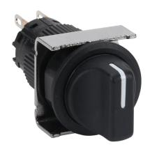
Fuji Electric selector switch, IP65, 19mm, 3-position, spring return to center from left, maintained right, DPDT contact(s), plastic base, plastic bezel, Operator: black, knob, 22mm, round, plastic.
