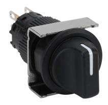
Fuji Electric selector switch, IP65, 19mm, 3-position, maintained, DPDT contact(s), plastic base, plastic bezel, Operator: black, knob, 22mm, round, plastic.
