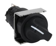
Fuji Electric selector switch, IP65, 19mm, 2-position, maintained, SPDT contact(s), plastic base, plastic bezel, Operator: black, knob, 22mm, round, plastic.
