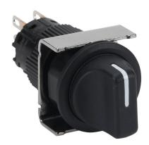
Fuji Electric selector switch, IP65, 19mm, 3-position, spring return to center from right or left, DPDT contact(s), plastic base, plastic bezel, Operator: black, knob, 22mm, round, plastic.
