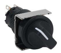
Fuji Electric selector switch, IP65, 19mm, 2-position, spring return from right, DPDT contact(s), plastic base, plastic bezel, Operator: black, knob, 22mm, round, plastic.
