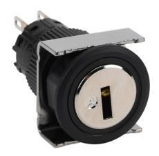
Fuji Electric selector switch, IP65, 19mm, 3-position, spring return to center from right, maintained left, key removable left and center position, DPDT contact(s), plastic base, plastic bezel, Operator: silver, key, 22mm, round, metal.
