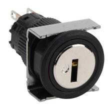
Fuji Electric selector switch, IP65, 19mm, 3-position, spring return to center from right, maintained left, key removable center position, DPDT contact(s), plastic base, plastic bezel, Operator: silver, key, 22mm, round, metal.
