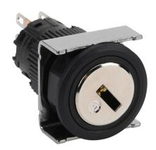
Fuji Electric selector switch, IP65, 19mm, 3-position, spring return to center from right, maintained left, key removable left position, DPDT contact(s), plastic base, plastic bezel, Operator: silver, key, 22mm, round, metal.
